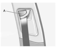
Move the height adjuster up to the desired position by pushing up on the height adjuster.
